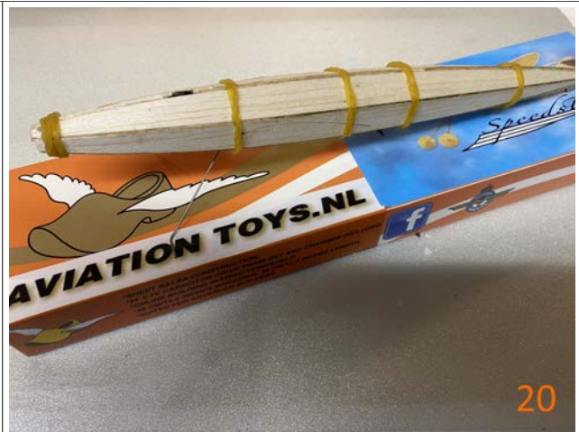
20. After glueing all 6 fuselage parts into place you can use rubber bands to keep it all in place while drying.
