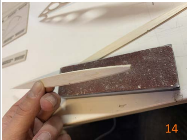
14. Before we can glue these bottom sheets into place, we have to sand the edges into a angle so the sheets fit without any gaps in between. take care in this process and try not to sand so much that you change the outline of the sheet. This process is needed for all 6 sheet fuselage parts.
