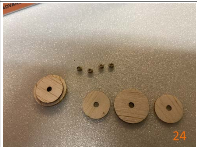
24. Wheels. Each wheel is made from one big and two smaller parts. Glue these together and sand them.
