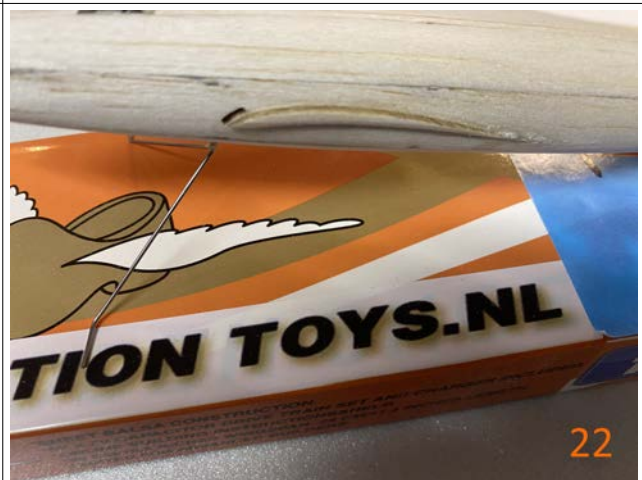
22. Glue the "airfoil-formers" into their position. There is a guiding line which still can be seen after sanding, Take extra care to glue left and right formers in the correct place.
