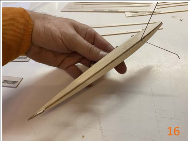
16. Make sure there is no gap between the sheet bottom parts and the center fuselage part.
