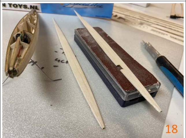
18. Top fuselage parts, take notice the part with the notch in it is for the right side.
